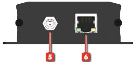
5. **Latch-locking power jack:** Connect to 12V DC power supply
