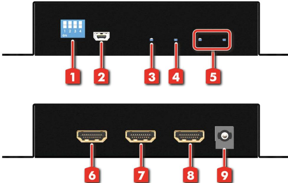
1. **EDID MODE:** See more detail in the DIP SWITCH SETTING section
